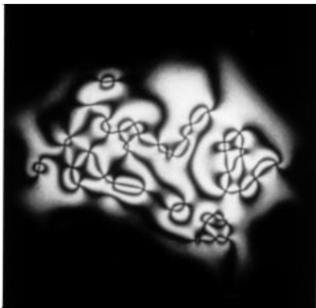
Figure 6. Schlieren texture of polymer PC6A (photograph taken at room temperature).
